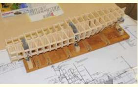
Paul Hines - An ambitious scratchbuilding work in progress, a 1/40 scale all wood plank on frame model of a modern 80 foot US Coast Guard cutter from Taubman Plan Service 1/48 scale plans, rescaled at Seneca Blueprint. Currently the keel and frames are assembled, getting ready for planking.
